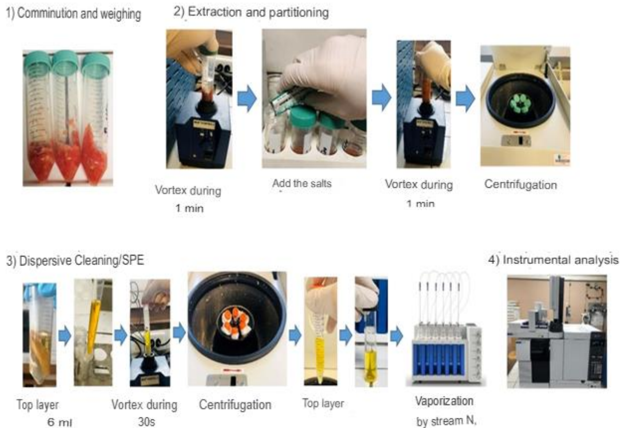
Figure 14: Simplified diagram of the process (Original photo).
