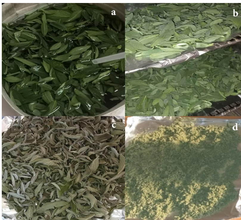
Figure 07: Sample preparation procedure; a) Cleaning leaves, b) oven drying of leaves, c) Dried leaves; d) leaf powder.
