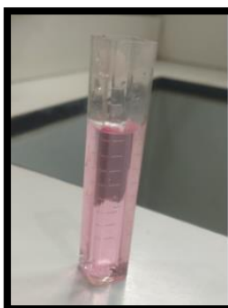
Figure III.17: Test de chlore positif.
