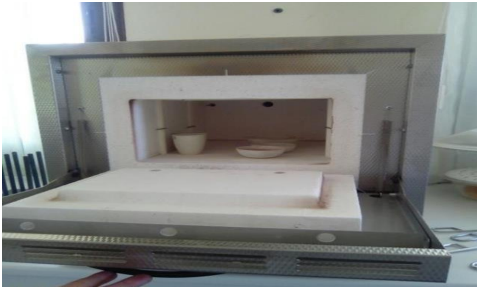
Figure III.14: Four à moufle ( 550\text{°C} )
