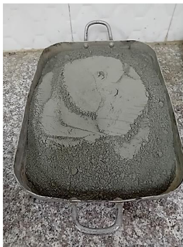
Figure III.1. Ciment (CEM I 42.5 N SR3 LH de BISKRA)
