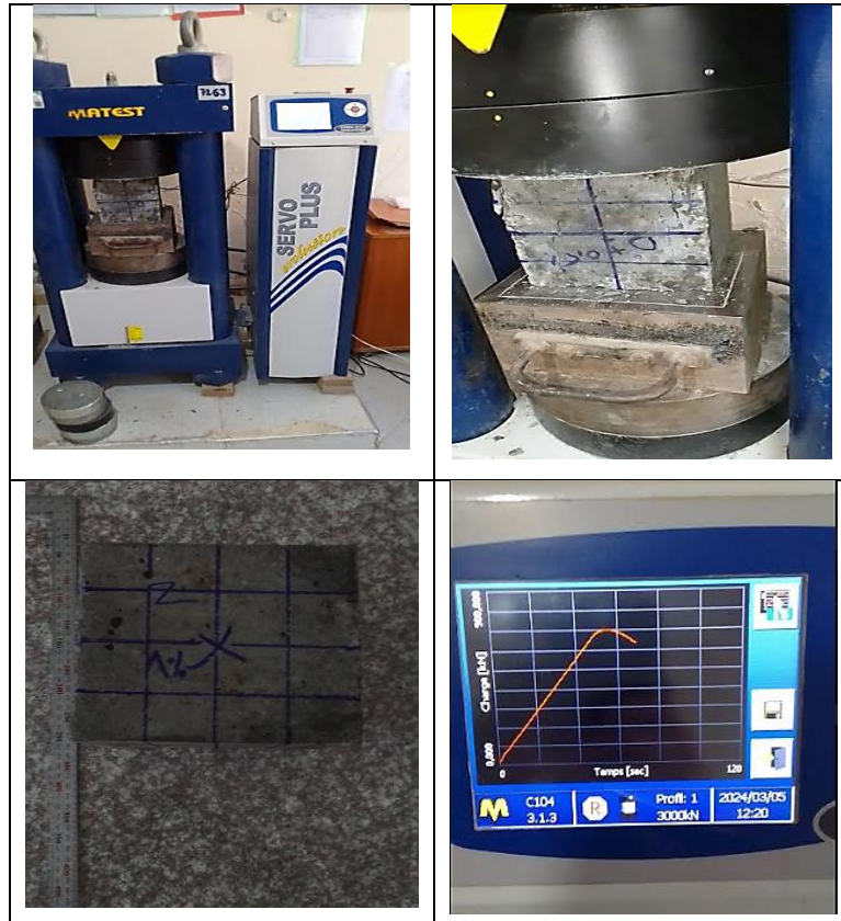
Figure III.18. Essai de compression a 7 jours
