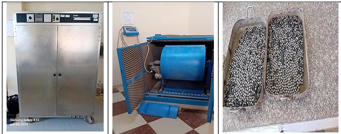
Figure III.10. Essai de LOS ANGELES
