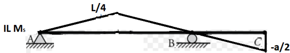
Figure 3.4 : influence lines of bending moment at Section S
