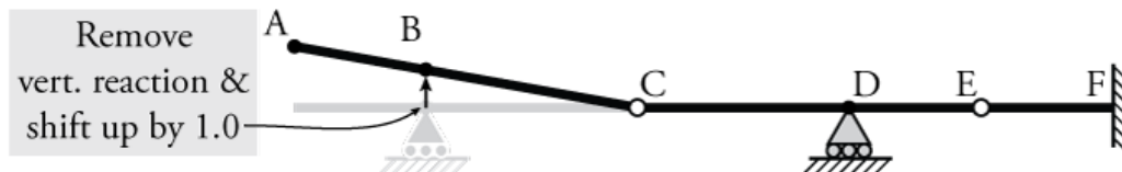
Figure 3.8 : the process for the determination the influence line for the vertical reaction at point B
