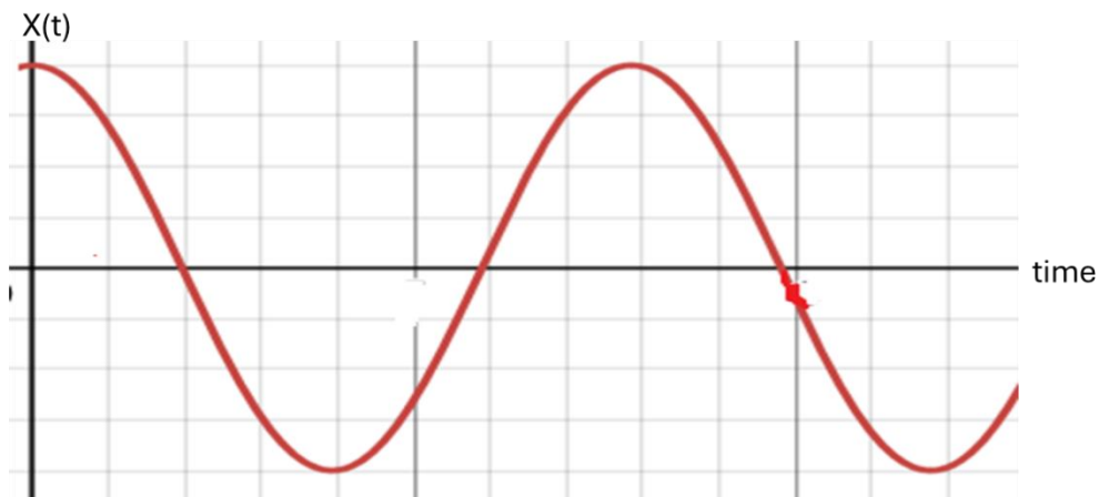
Fig.3: the graph illustrating the curve of the simple harmonic motion
