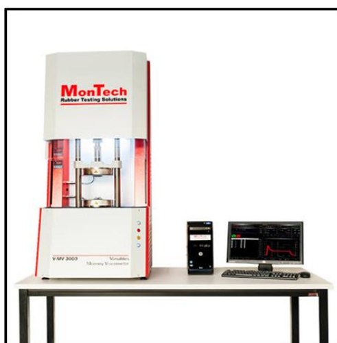
Figure III.14: Mooney viscometer machine [44].
