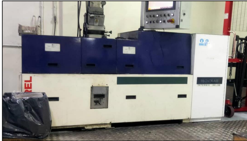
Figure III.2: TECHNOLAB mixer (intermix IM 1.5E).
