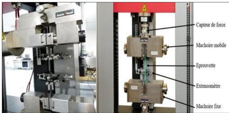
**Figure III.13.** Machine de la traction.
