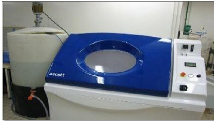
Figure II.15. Brouillard salin.
