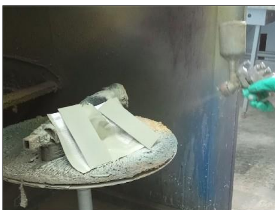
Figure II.10. Application de Phosphale.
