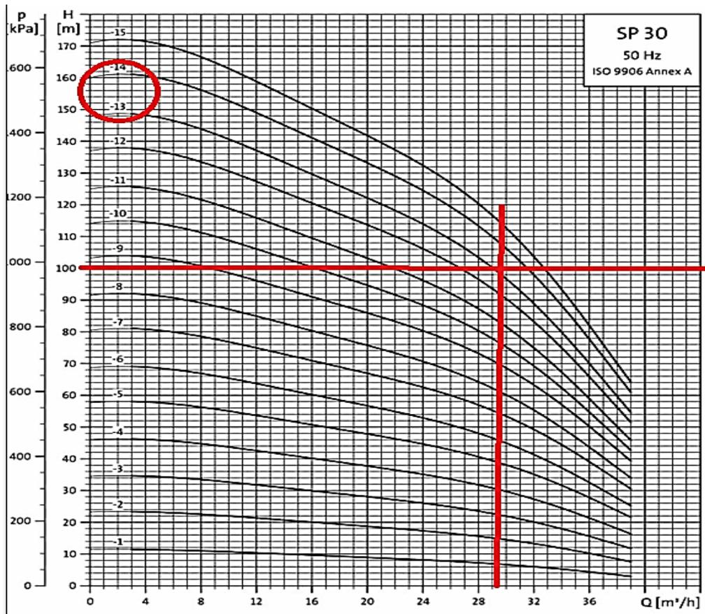
Figure III. 6: Abaque de la pompe SP 30 [6]
