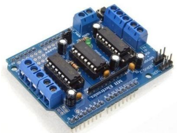
Figure II.5: image montre un Module L293D [39].
