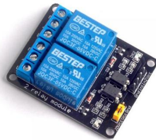
Figure II.6: image montre un Module Relais 5V, 2 Canaux [40].
