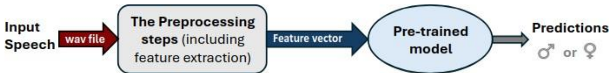
Figure 3.28 : Architecture of the Real-Time Gender Classification system
