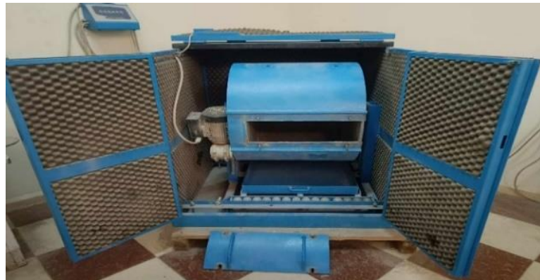
Figure III.8. Essai Los Angeles
