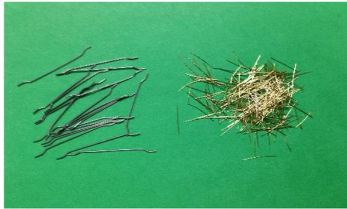
Figure II.5. Types des fibres (Crochet et Droite)
