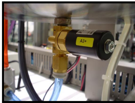
FIGURE VI. 11: VANNE DE REGULATION ELECTRIQUE.
