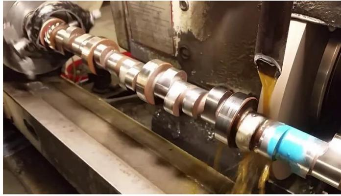
*Figure.I.10: A Camshaft*
