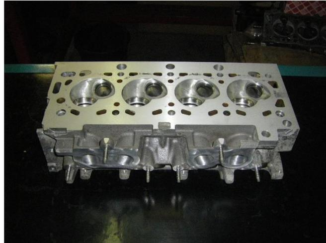
*Figure.I. 4:* Aluminium cylinder head
