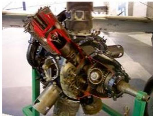
*Figure.I.21:* a Radial/Star Engines
