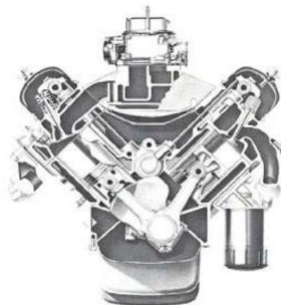
*Figure.I. 18 :* An engine with 'V' shape
