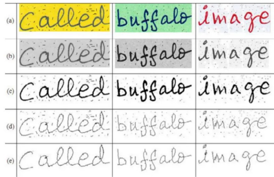
FIGURE 2.3 – (a) Original Image. (b) Converted to Grayscale. (c) Binarized image. (d) Thinning and Skeletonization are done. (e) Noise Removed[6]
