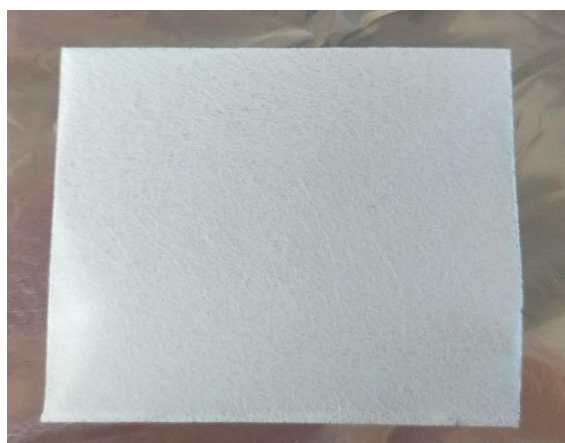
Fig. S4. \text{TiO}_2 coated GFT ( 25 \text{ cm}^2 )
