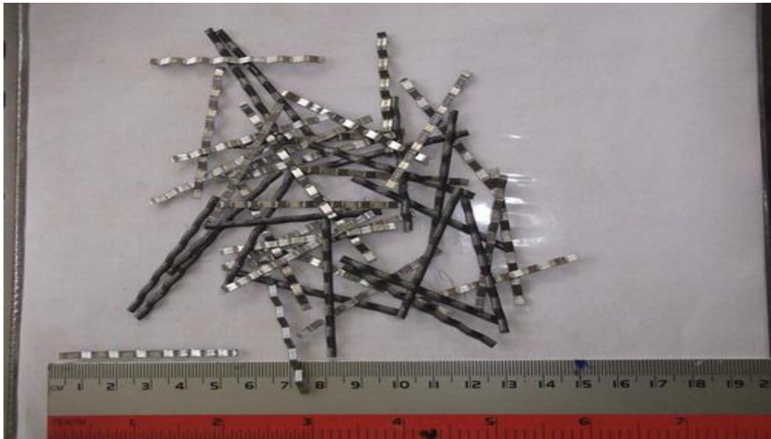
Figure 1. 8 Fibres d'acier Embouties [38].
