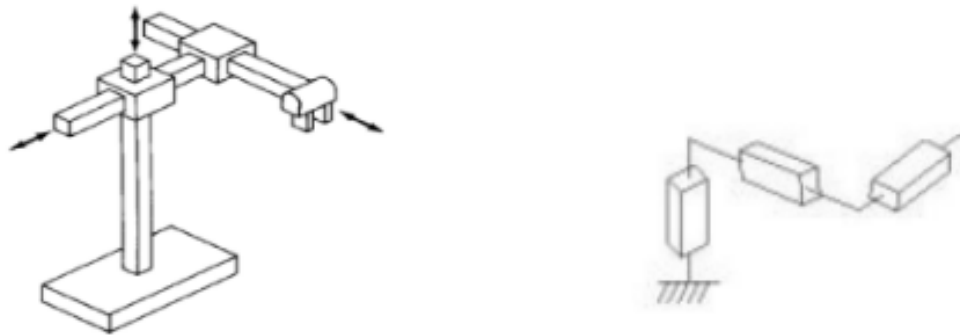
Figure 1-18: Structure cartésienne
