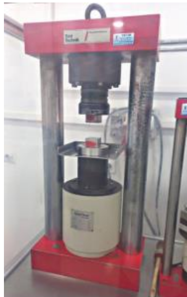
Figure II.10 : Essai de compression
