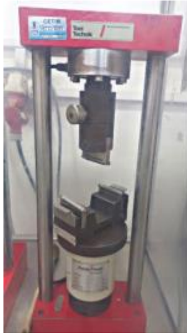
Figure II.9 : Essai de Flexion
