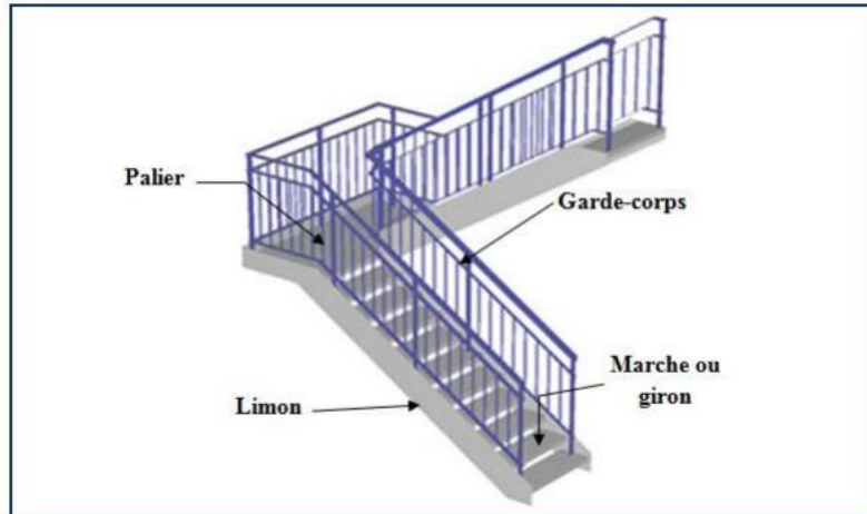
FIGURE V 1 The elements of a staircase.
