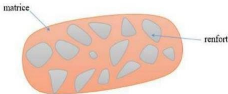
Figure I. 1: Constituent d'un matériau composite [02].
