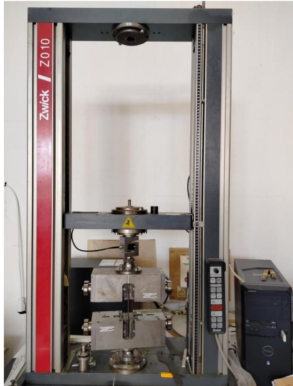
Figure II - 24: machine de traction Zwick/Roell.
