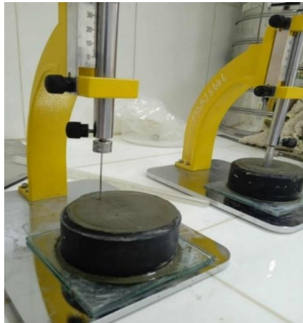
Figure II - 9: Essai de prise.
