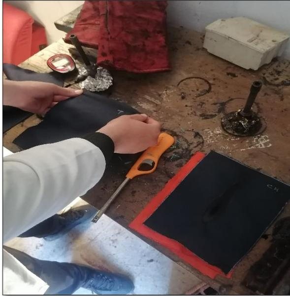
Figure III-8 : Frame for mounting specimens.
