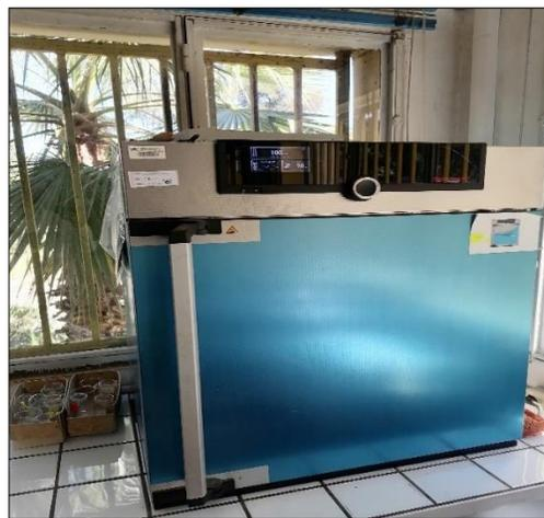
Figure III-3 : Drying oven NUIVERSEUE OVEN 108 MEMME
