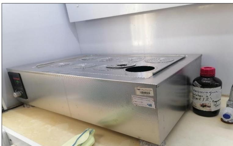
Figure III-5 : Water bath 29L stainless steel with temperature control
