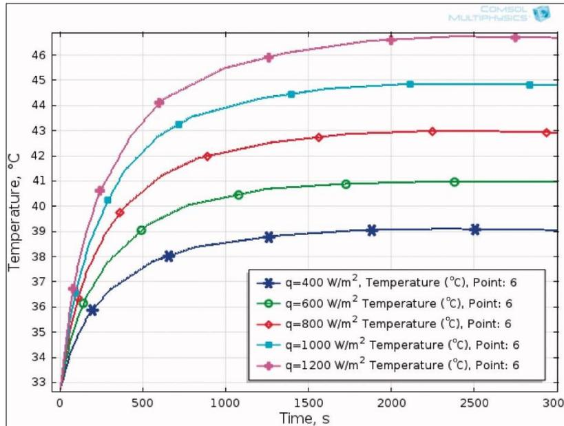
Figure II-7 : Influence of the heat flux on the temperature of the basal layer for a three-layer system and 1-mm air gap between the fabric and the skin. [98]
