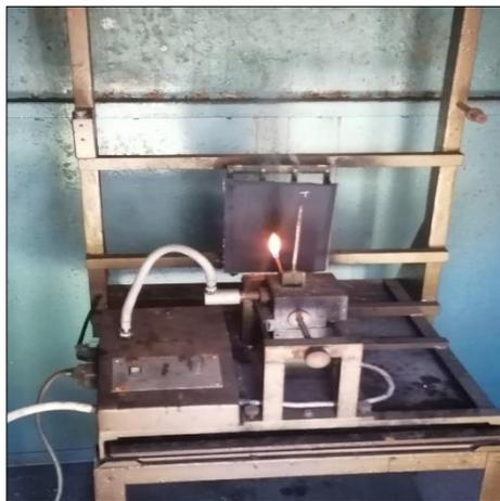
Figure III-7 : Flammability tester.
