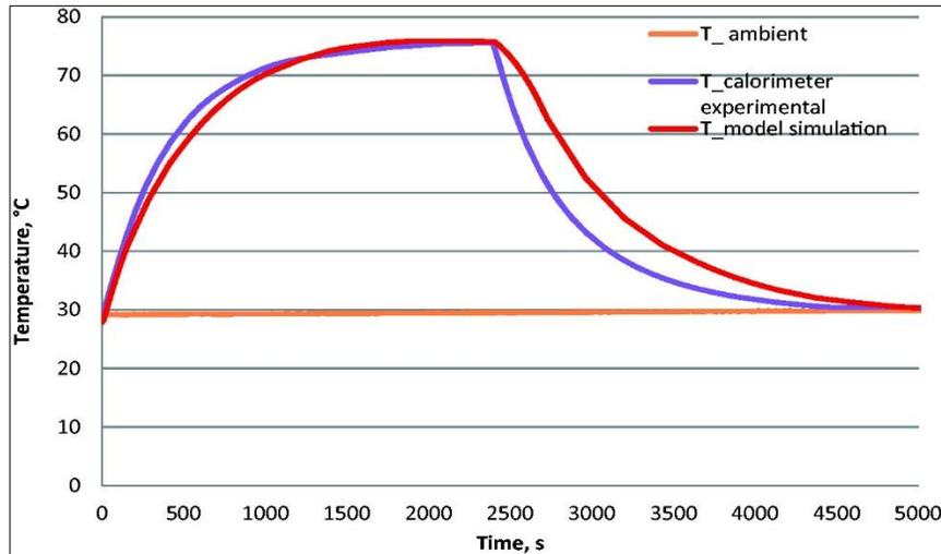
Figure II-6 :Comparison of computational and experimental results of calorimeter temperature for a three-layer system and 1000 W/m<sup>2</sup> inward heat flux.
