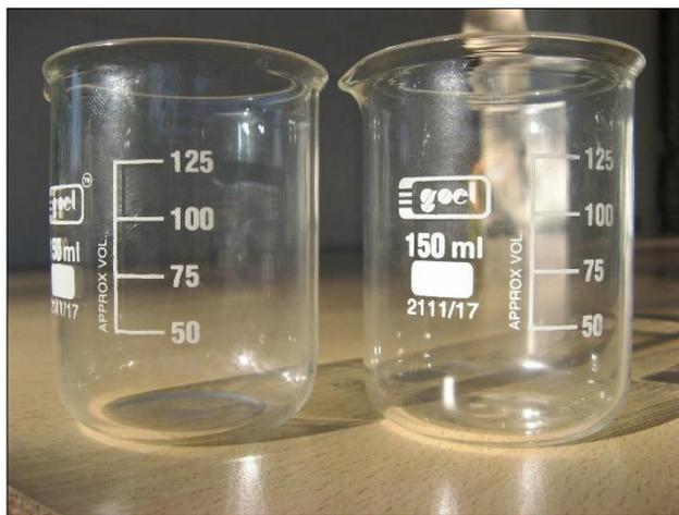
Figure III-6 : Beakers Borosilicate glass
