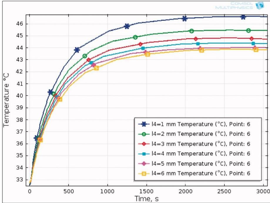
Figure II-8 : Influence of the air gap width on the temperature of the basal layer for a three-layer system and 1200 W/m<sup>2</sup> inward heat flux. [101]
