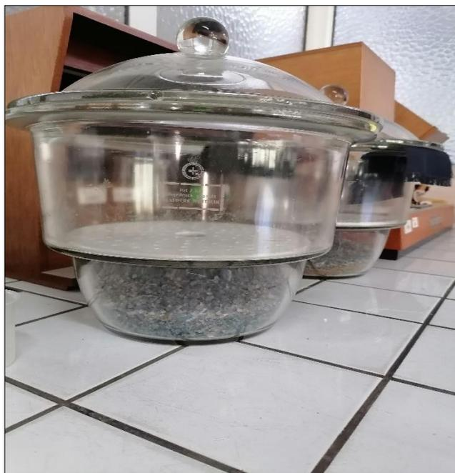
Figure III-4 : Desiccator Standard glass desiccator with silica gel
