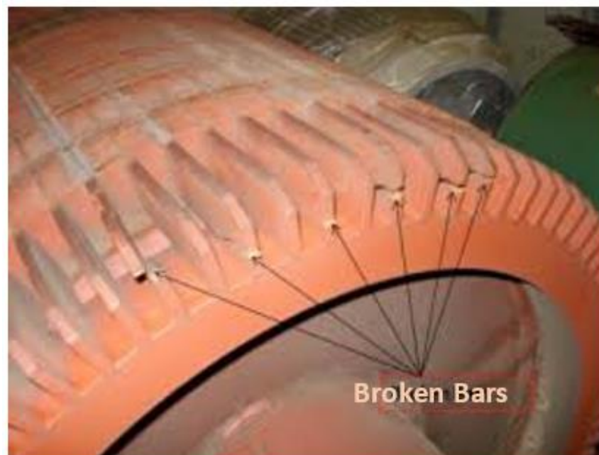
Fig I.15 Broken rotor bars.
