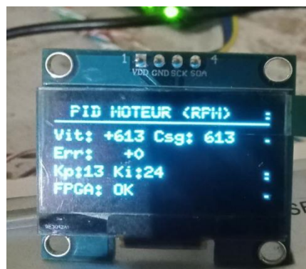
Figure IV.10 — Affichage OLED via Arduino Uno (relais UART)
