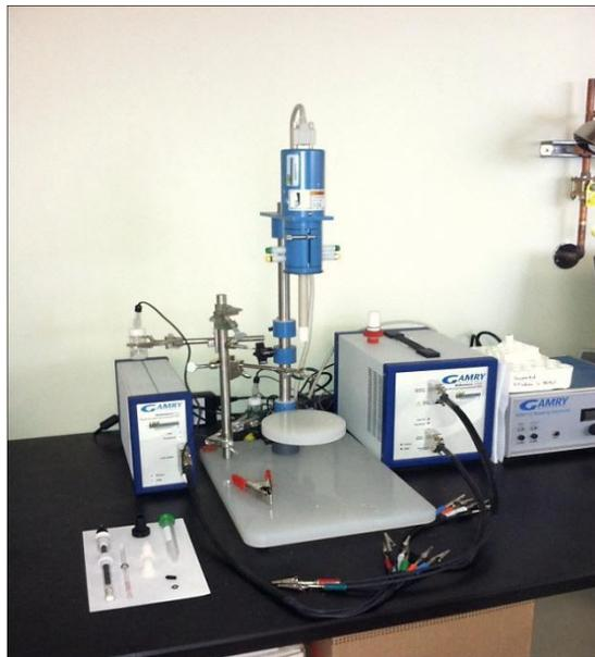
**Figure III-8:** Potentiostat galvanostat ZRA GAMRY reference 3000.
