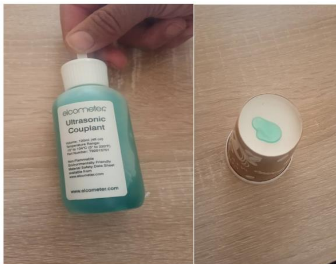
Figure II.7 Liquide couplant ultrasonique. [20]
