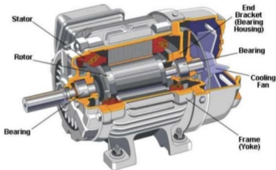
Fig. I.6: Construction of an Induction Motor [13]
