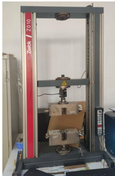
Figure III.1: la machine universelle (ZwickRoelle)
