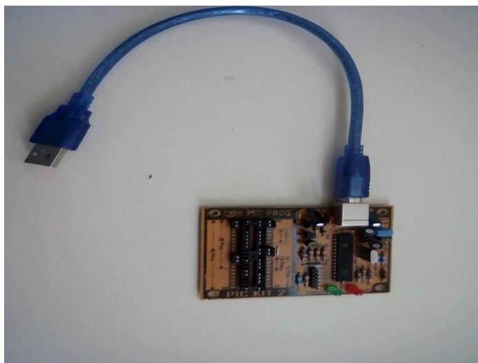
Figure 2.19. USB ICSP PIC programmer et ICSP PIC programmer socket
