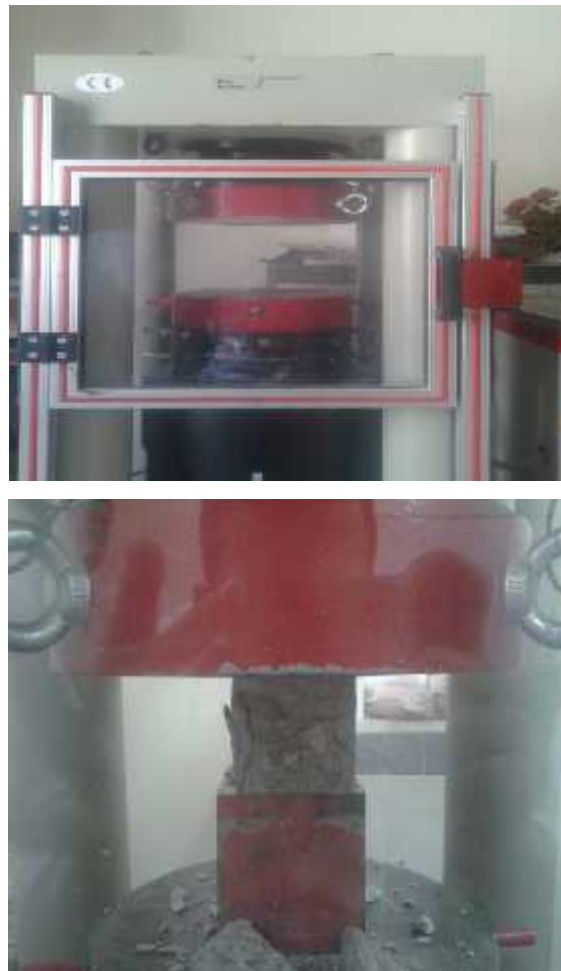
Figure 60: Essai de compression
