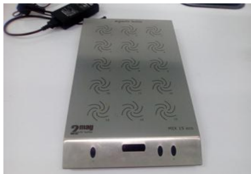
Figure 15 : Agitateur (2mag-magmatic motion-MIX 15 eco).
