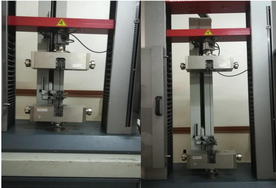
Figure III.9: Machine de traction.
