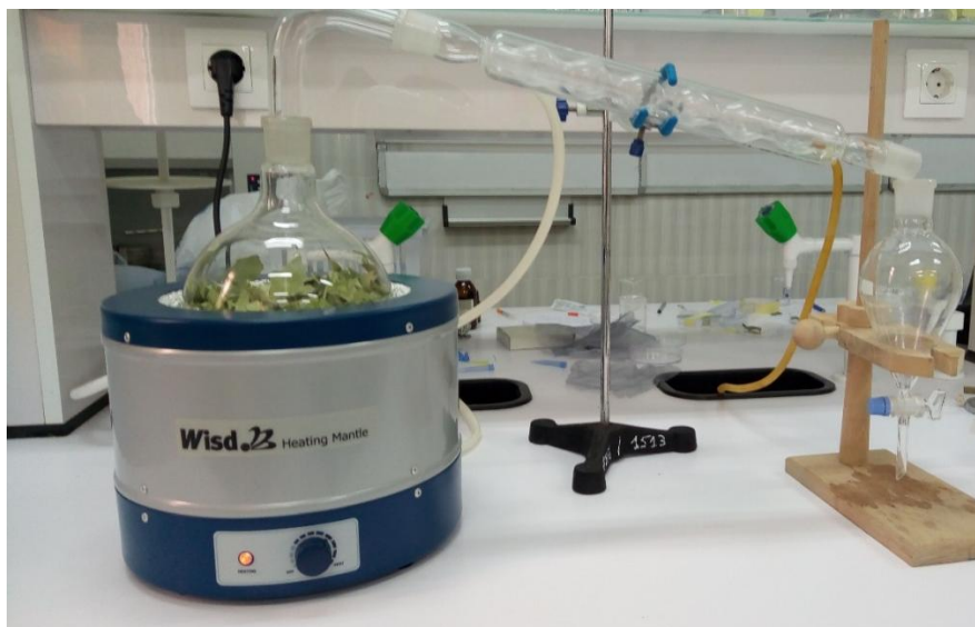
Figure 12: Montage d'hydrodistillation (Clevenger) (original).
