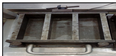
Figure II. 17: Le moule prismatique (40x40x160) mm.
