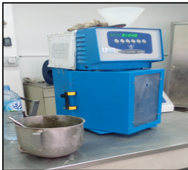
Figure II. 18: Malaxeur. Figure II. 19: Table à choc. Figure II. 20: Aplanir les moules.
