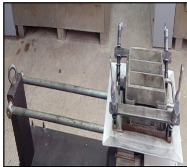
Figure II. 18: Malaxeur. Figure II. 19: Table à choc. Figure II. 20: Aplanir les moules.
