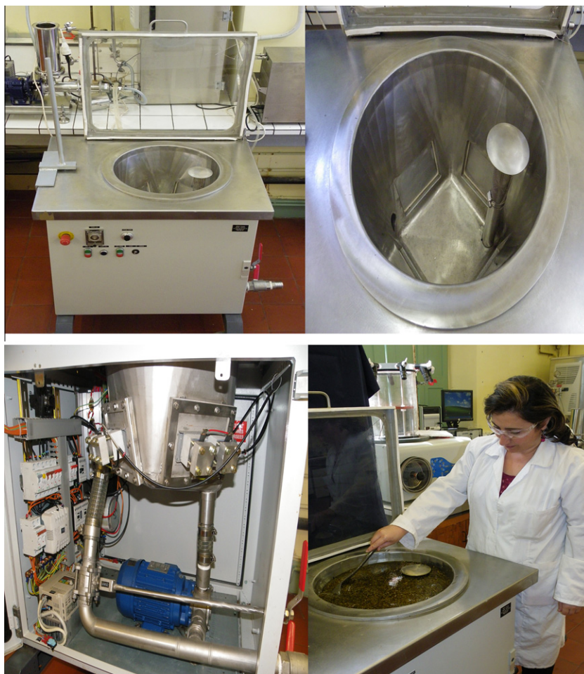
Fig. 8. Pilot plant ultrasonic device (30 L) used for ultrasound-assisted enrichment.
