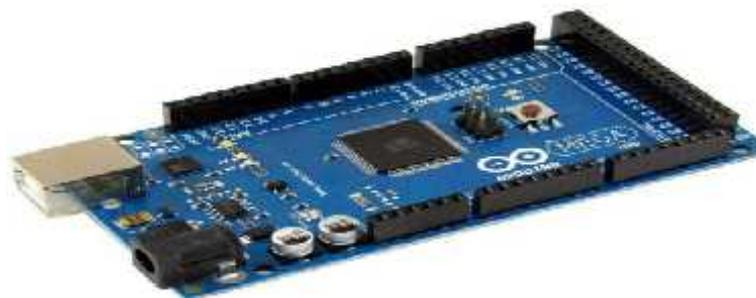
Figure (4.1) : Arduino Mega 2560 [14].
