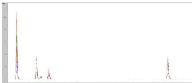
**Fig. 1** – Chromatograms of a series of standard calibration solutions with the following order of elution: ascorbic acid (1.6 min), thiamine (2.3 min), pyridoxine (2.5 min), nicotinamide (2.8 min), ribofavin (6 min)
