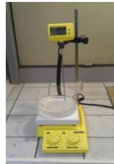
(b) The beaker, samples and SBF during heating and stirring
