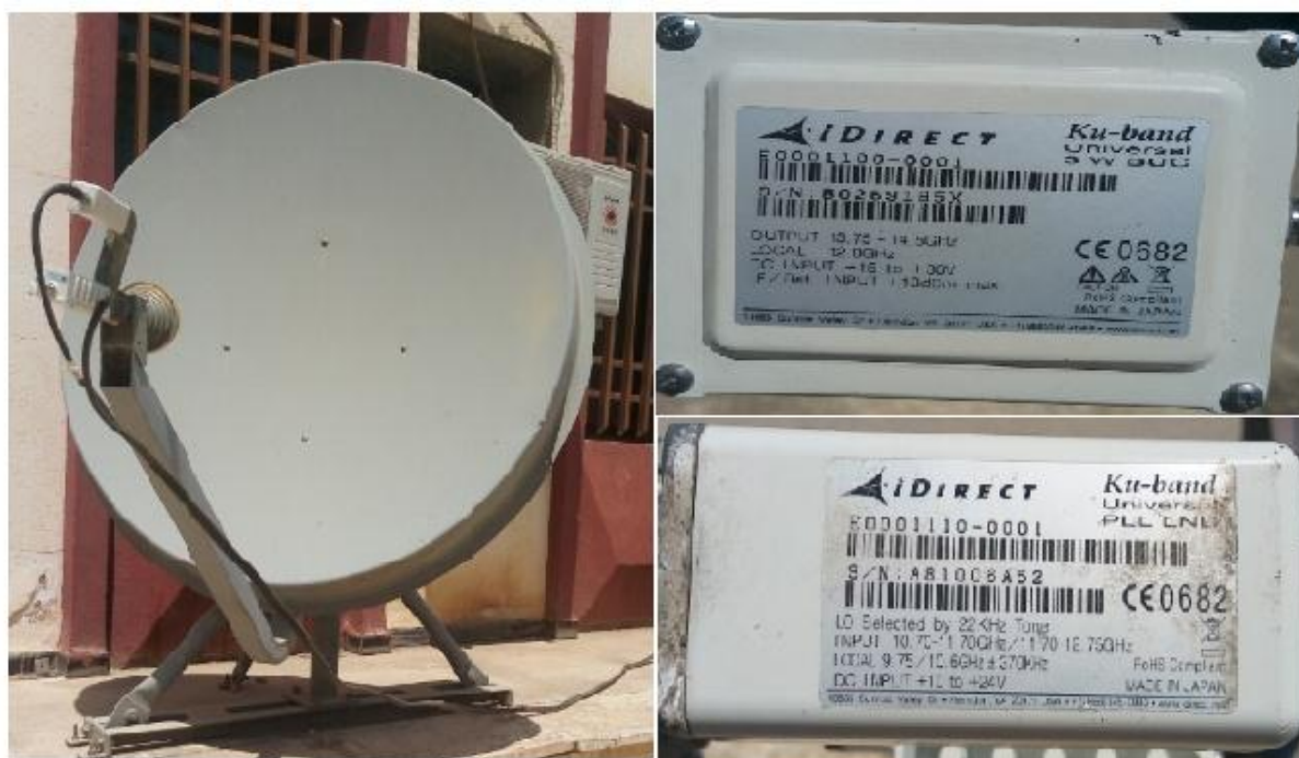
Figure III.14 : Antenne, LNB, BUC.
