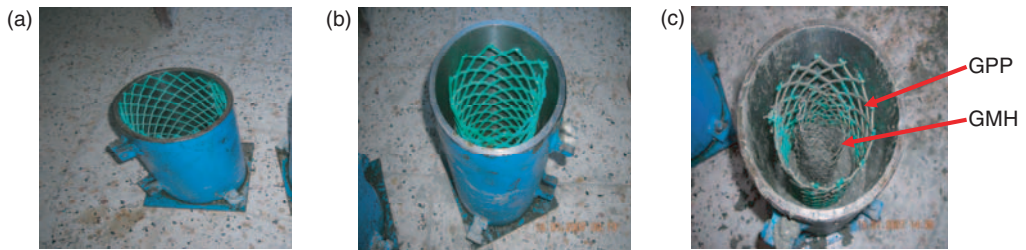
Figure 2. Examples of grid arrangements: (a) exterior grid, (b) interior grid, (c) hybrid grid.
