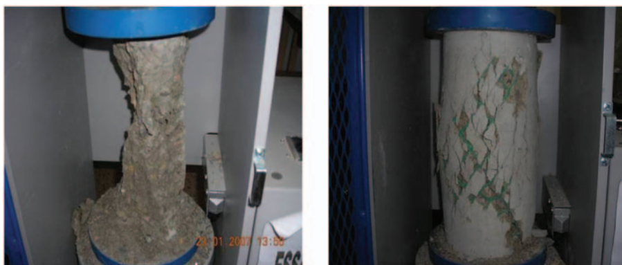
Figure 9. Mode of rupture of the reference concrete and confined concrete.
