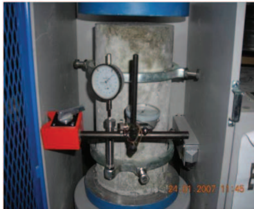
Figure 3. Measurement devices and loading of the specimens.
