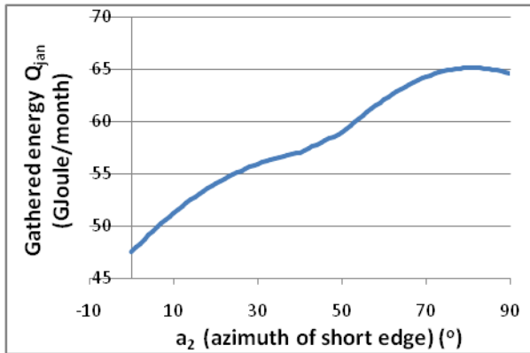
Figure 4: Amount of gathered solar energy by greenhouse versus change of a_2 in January
