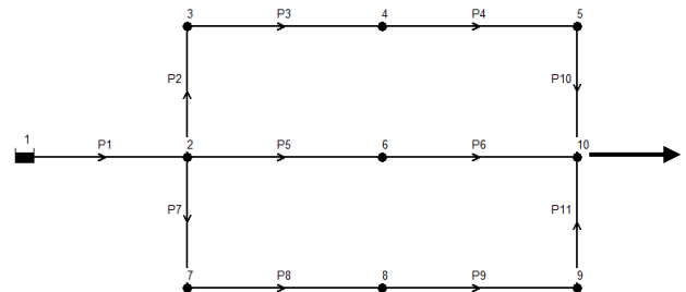
Figure 1: Simple pipe network (Aggregation level 1).
