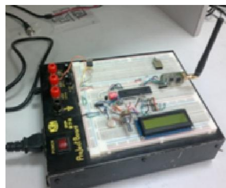
Figure 8: Testing a node on a project board
