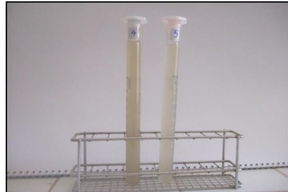
Figure 7: Utilization of polluted water to visualize the change due to ozone (4 before and 5 after).
