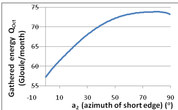
Figure 13: Amount of gathered solar energy by greenhouse versus change of a_2 in October
