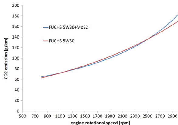
Fig. 10. Engine rotational speed versus CO 2 emission factor curves obtained from constant speed cycle data.
