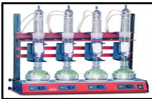
Figure II.1 : Extraction au soxhlet.
