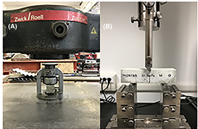
FIGURE 2 Mechanical tests: a) compression test - b) flexural test
