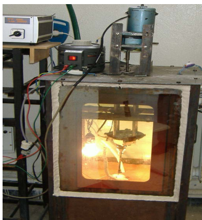
Figure 1. Homemade heater used for monocrystalline synthesis.
