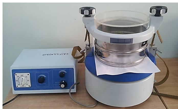
Figure II.13. Schéma de tamiseuse type JINLING.
