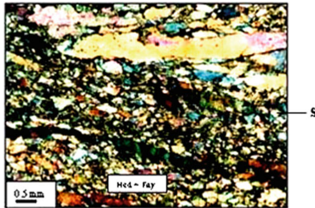
Fig. 5 Silicate ore from Berrahal iron formations. El Mour Ouan'ya mine. Hed: Hedenbergite; Fay: Fayalite. Thin section, crossed nicols view
