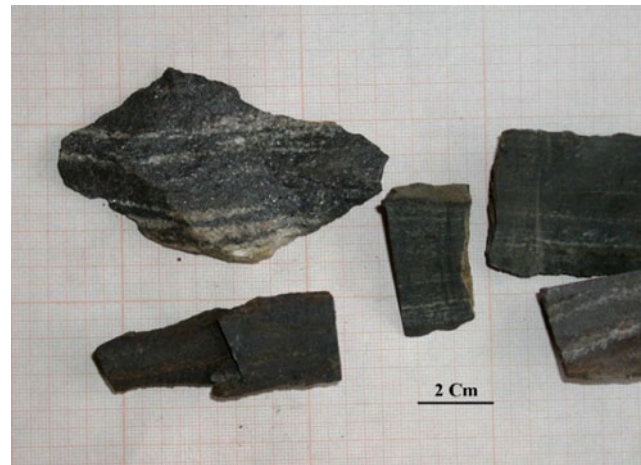
Fig. 4 Metamorphic bands of carbonate ore (alternation of iron oxides (dark) bands and carbonates (light) bands)
